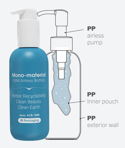
(For the PP pump, the spring remains metal for reliable performance.)
